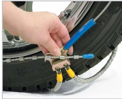
**5** Repeat this process with the gold adjustment fastener. Ensure that both fasteners are adjusted within one bead of each other. Move the vehicle a few feet. Remove cable "slack" by retightening both adjustment points as equally as possible.
