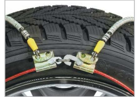
**3** Reach around each side of the tire and grasp both ends of the non-split side cable (that is furthest away from you). Pull both ends to the top of the tire so the fasteners can be seen and manipulated more easily. Connect the inside fastener.
