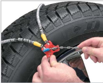
**4** Grasp the outside cable with both hands and pull it toward you to create as much slack as possible. Connect the top fastener (the red one) as tightly as possible by inserting the silver "beads" on the cable through the keyhole.
