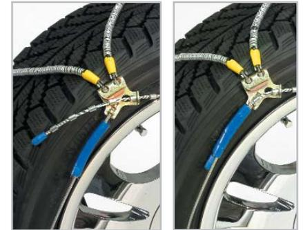
**6** To secure the free ends of the cable, slide the plastic spirals over them with a twisting motion. If insufficient cable is available for plastic spirals to secure, "tuck" the short end up next to the cross member anchor points, as shown.
