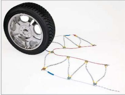
**1** Park vehicle on firm, level ground and away from the flow of traffic. Set the emergency brake. Chains should be installed on drive wheels. Lay the cable chain on the ground with the smooth side (TIRE SIDE) of the crossmember hooks up.
