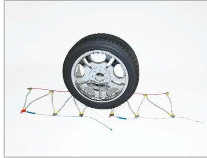
**2** Move the chain in a sweeping motion under the vehicle so the open mid-section is positioned up against the backside of the tire. This sweeping motion can best be done while kneeling in front of the tire.
