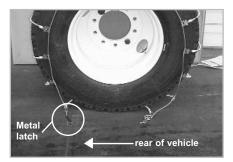
Drape the chain over the top of the tire so both ends can touch the ground and the long metal latch is on the outside of the tire (toward you) and is draped toward the back of the vehicle. The two half sets are made so that one fits only on the left and one only on the right. See Close-up below
