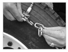
Connect the "speed hook" on the inside of the tire (the side away from you). As a starting point, we recommend that you fasten it so that there are no more than two "free" links. It may be necessary to drive forward two to three feet so that the inside connection can be made more easily.
