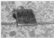
Make sure that the smooth side of the eyelets (marked "TIRE SIDE") are against the tire. If the smooth side is not toward the tire, damage will occur.
