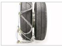
Keep the cable chain folded and drape it over the top of the outside tire. Both side cables are at the front of the tire.
