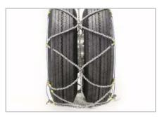
Flip top half of the chain over the top of the inside tire. Make sure that the smooth sides of the eyelets (marked "TIRE SIDE") are against the tire.
