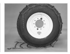
Drive forward a few feet, far enough so that two or three of the cross chains pass under the tire.
