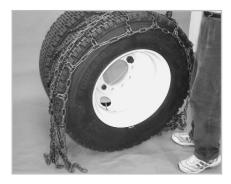
Park vehicle on firm level ground, and turn off the engine. Set the parking brake. Lay the chains out flat on the ground, making sure there are no twists or tangles. Make sure the cross chain hooks are facing upward. Drape the chain over the tire, so that one cross chain is postioned at the point where the tire meets the ground.
