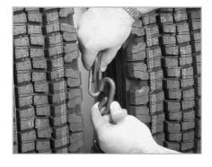
Reach behind the tire and engage the inside connector making sure it is as tight as possible. See the illustration below for a detailed look at this connection.
