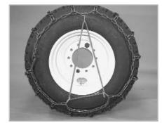
SCC recommends chain tighteners (sometimes known as chain spreaders) be used to take up additional slack. To make this simpler, attach the first hook at the "11 o'clock" position, the next at the "5 o'clock" postion and so forth. The open side of the hooks must face away from the tire. No further adjustment should be necessary.
