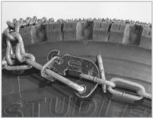
Next fasten the outside fastener, again making sure it is as tight as possible. Drive a short distance and retighten all fasteners. For best results, make sure all connections are equal and as tight as possible.
