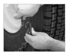
Reach behind the tire and fasten the inside connector making sure it is as tight as possible. See the illustration below for a detailed look at this connection.
