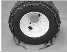
Drape the chain over the tire, so that one cross chain is positioned at the point where the tire meets the ground. Again make sure the cross chain hooks are facing upward. Hooks that face down (towards the tire) will cause damage to the tire. "CAM" side adjusters should be on the outside of the tire.
