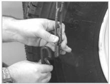
Next fasten the outside fastener in the same manner, again making sure it is as tight as possible. Drive a short distance and retighten all fasteners. For best results, make sure fasteners are adjusted equally and as tight as possible.
