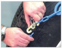
Next fasten the outside fastener, again making sure it is as tight as possible. Drive a short distance and retighten all fasteners. For best results, make sure fasteners are adjusted equally and as tight as possible.
