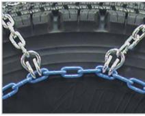
Again make sure the cross chain hooks are facing upward. Hooks that face down (towards the tire) will cause damage to the tire. "CAM" side adjusters should be on the outside of the tire.
