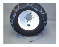
Park vehicle on firm level ground and turn off the engine. Set the parking brake. Lay the chains out flat on the ground, making sure there are no twists or tangles. Make sure the cross chain hooks are facing upward, then drape chain over the tire, so that one cross chain is positioned at the point where the tire meets the ground.
