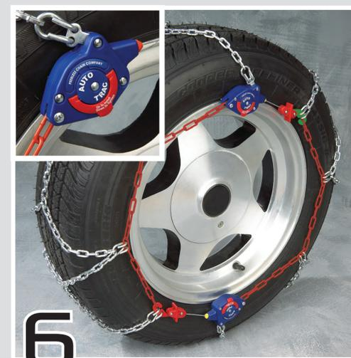
6. Flip the red lever down to tighten both the top and bottom tensioners. Your chains will begin to self tighten.
