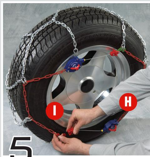
5. Grasp the bottom tensioner (H) and flip the red lever up to install. Pull the red cable end out and connect to the side chain connector (I). **PINCH WARNING:** Keep your fingers clear of the chain and tensioner while engaging the tensioners.
